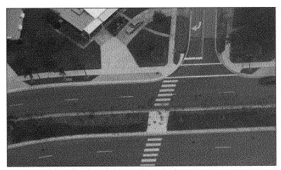
FIGURE 7-4. Refuge islands provide pedestrians with a resting place when crossing roads or intersections.
