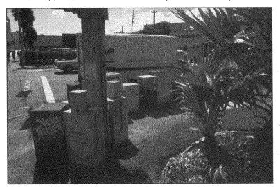
FIGURE 3–7(b). Sidewalks should be designed to be clear of poles and other objects.
