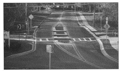
FIGURE 7–5. Cut-through ramps should be provided on refuge islands and medians to accommodate wheelchair users.
