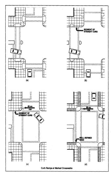
FIGURE 6-7. Guidelines for crossing placement at intersections.<sup>6</sup>
