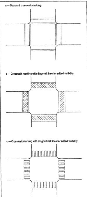
FIGURE 6-1. Typical crosswalk markings.'
