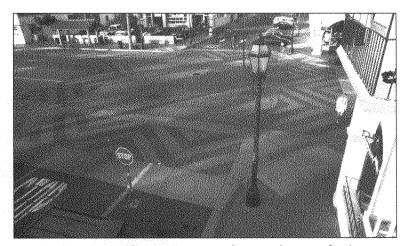
FIGURE 12–10. Raised intersections can enhance pedestrian safety by reducing traffic speeds.
