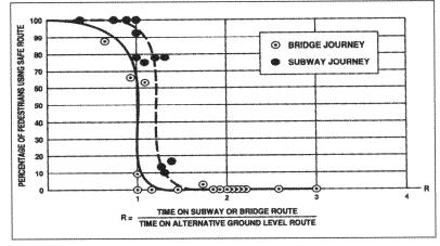
FIGURE 10-4. Pedestrian use of grade separated crossing.
