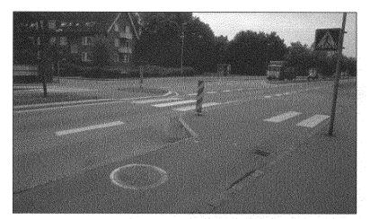
FIGURE 12–6. A choker is a narrowing of the street, either at an intersection or midblock, in order to reduce the width of the traveled way.
