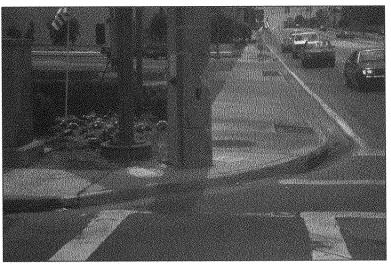
FIGURE 3-7(a). Sidewalks should be clear of poles and other objects.
