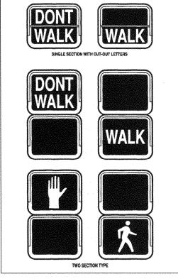
FIGURE 5-1. Pedestrian signal displays.<sup>1</sup>
