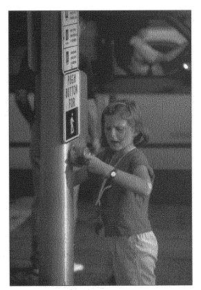
FIGURE 5–6. Pedestrian push-buttons are often provided at locations with intermittent pedestrian volumes to call for the WALK message and/or extend the crossing interval.
